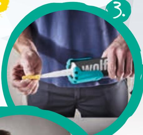
3. Insert your cartridge into a caulking gun. The MG 600 PRO is the ideal tool for this job because it can deliver extremely thick adhesives and sealants with ease.
