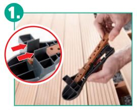
Positioning the joiners with the **drill and screw gauge** is child's play: Just put the joiner into the gauge from beneath.
