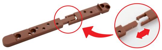
Fasten the deck board joiner with four screws underneath the board. It will automatically adjust for the wood's swelling and shrinking behaviour within its range of motion and thus prevent the formation of cracks and the screws from getting torn out.
