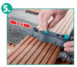
Adjust the front drilling bush with the help of the setting notch on the side in the same way, so that it hits the second marking line. You can now place the deck board in its correct position onto the supporting joists.
